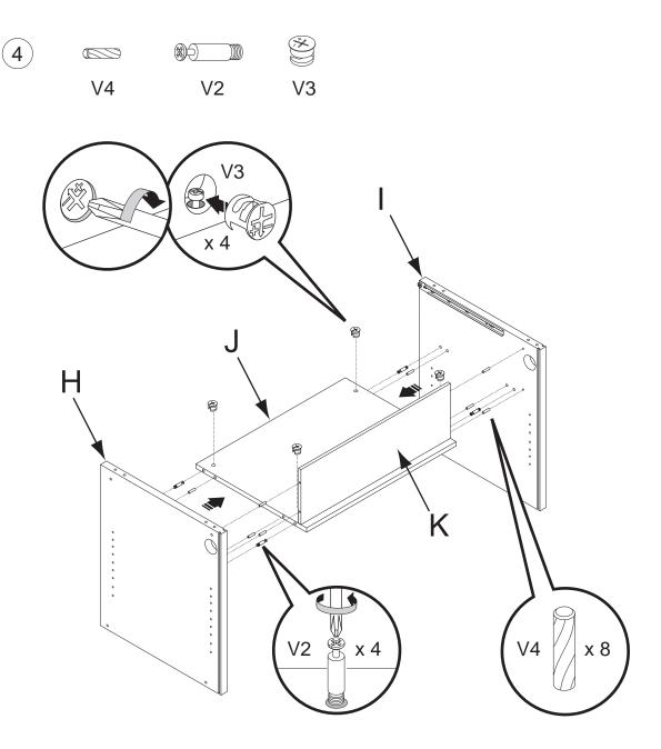
4. Attach Left & Right side board (H,I) to the middle boards (J,K) with screws (V2), cam lock(V3) and wooden dowels (V4),then turn cam lock(V3) clockwise to secure.
